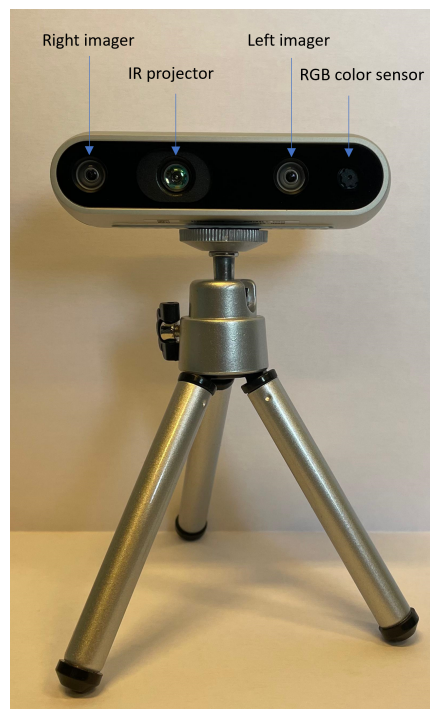
Figure A.1: The Intel ® RealSense ™ D435i camera and its imaging components.
