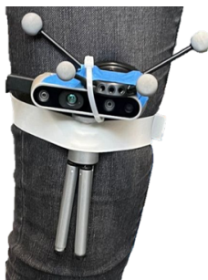
Figure 4.2: Attachment of the cluster of passive markers to the camera mounted on the knee.
