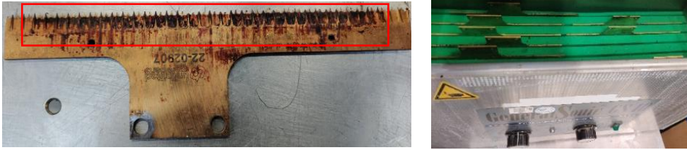
Figure 29 UBM – Dirt accumulation knife restoration task
