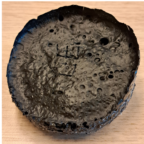
Figure 32: The prepared PLA/Fe 3 O 4 composite material with 100ml DCM, 33g PLA and 14.25g Fe 3 O 4 .
