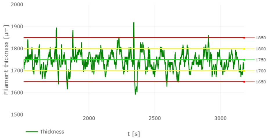
Figure 39: The measured filament diameter for the second filament making attempt
