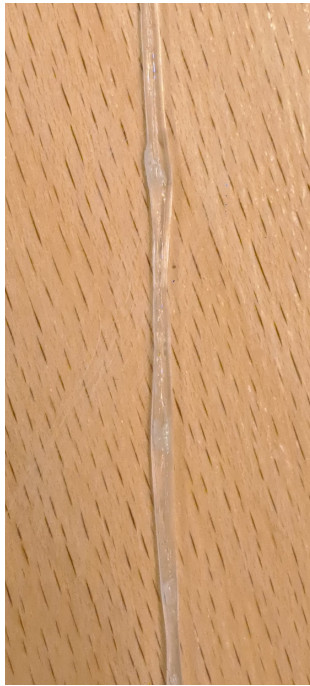
Figure 57: The cleaning material in PLA resulting in unstable diameter
