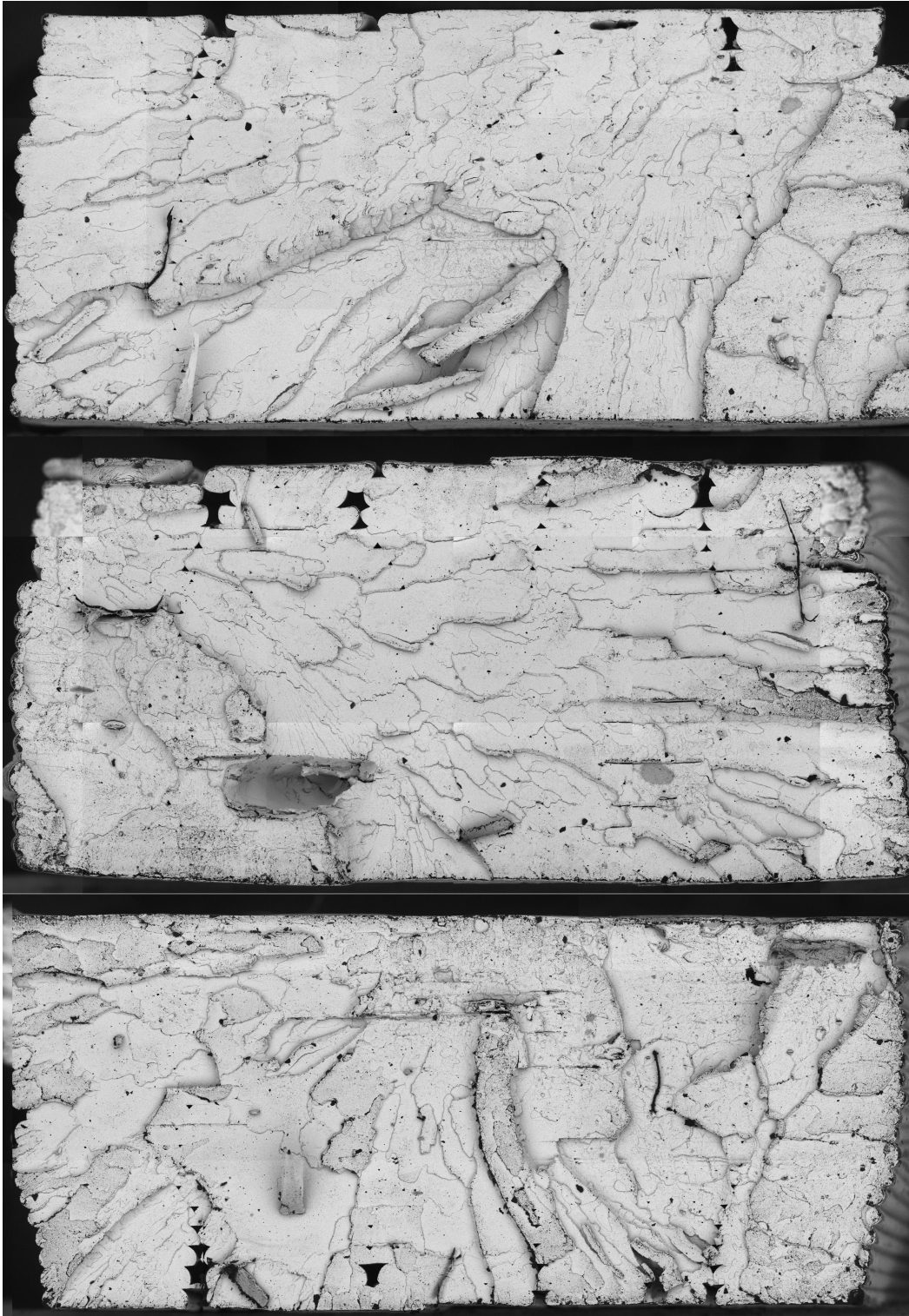
Figure 59: SEM images of complete fracture surface of PLA/Fe 3 O 4 composite material fractured with a tensile test
