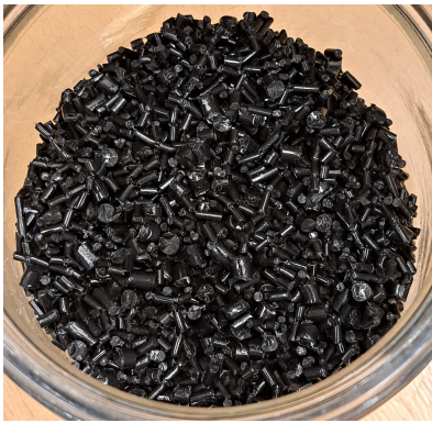
Figure 37: The cut filament prepared for the second filament extrusion
