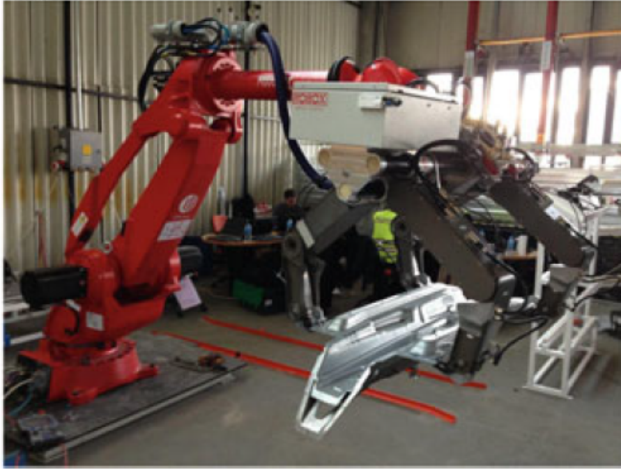
Figure 2.2: Reconfigurable fixture prototype [6]
