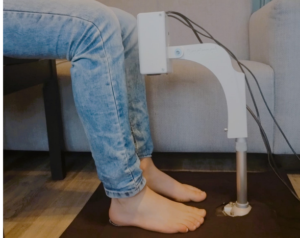
Figure 5: Set-up for measurement of the dorsal side
