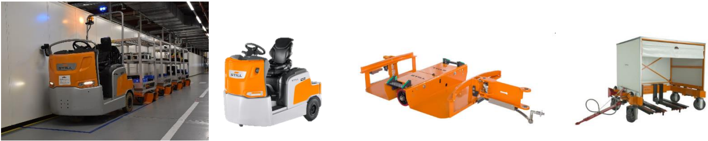
Figure 3 - Tugger train vehicles – Full, LTX70, B-Frame & C-Frame (Still, 2023)
