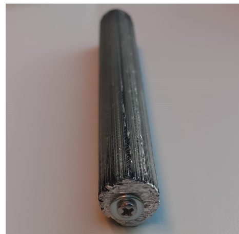
(b) Cylinder with conductive wires and 2 big bond pads with screws for connection.
