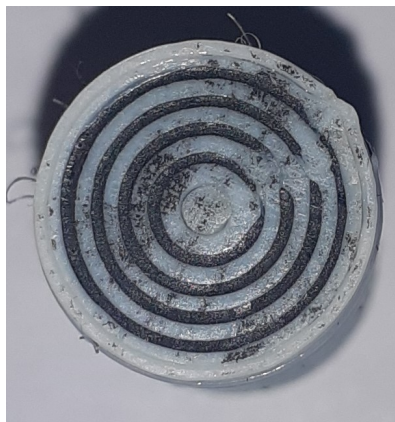
(a) Uncompressed cylinder made of NinjaFlex and PI-ETPU rings.
