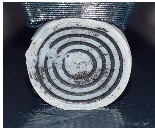
(b) Compression of a NinjaFlex cylinder with PI-ETPU rings to visualize the deformation.
