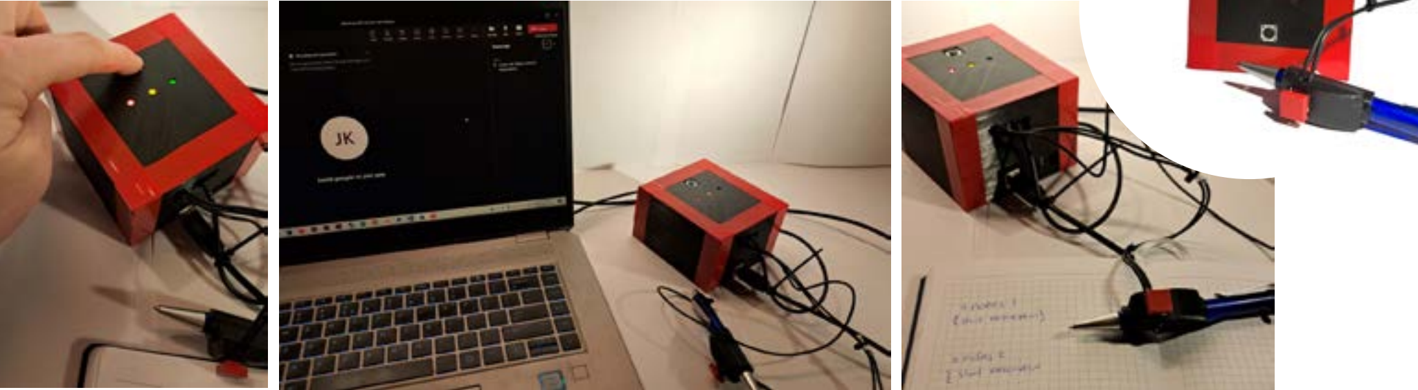
Figure 55: Functional marker prototype ideas integrating inputs into a pen and button board. The functionality of the pen prototype has been realized.
