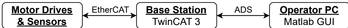
Figure 4.3: Schematic representation of the electronic systems used during operation of the exoskeleton, with the corresponding communication protocols.
