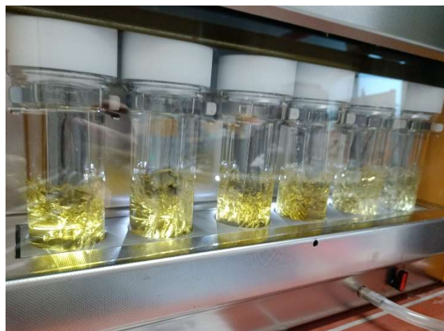
Figure 23: Extraction running in the Soxtherm extraction unit
