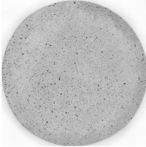
Figure 9: White rubber sample with clearly visible particles
