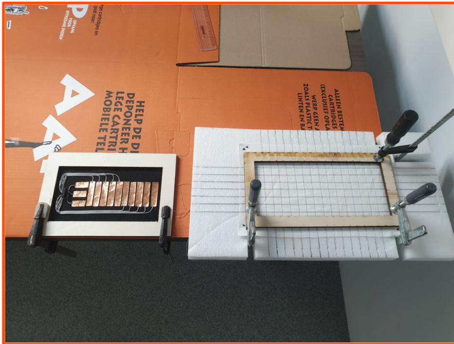
Figure 64: The final setup with the Trill prototype(left) and the MuCa prototype(right) without silicone
