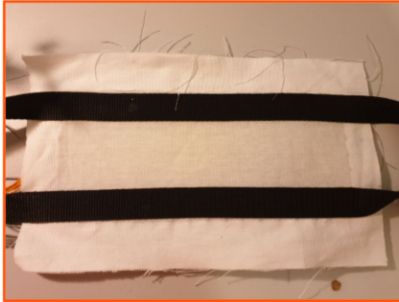
Figure 78: silicone MuCa module with nylon straps
