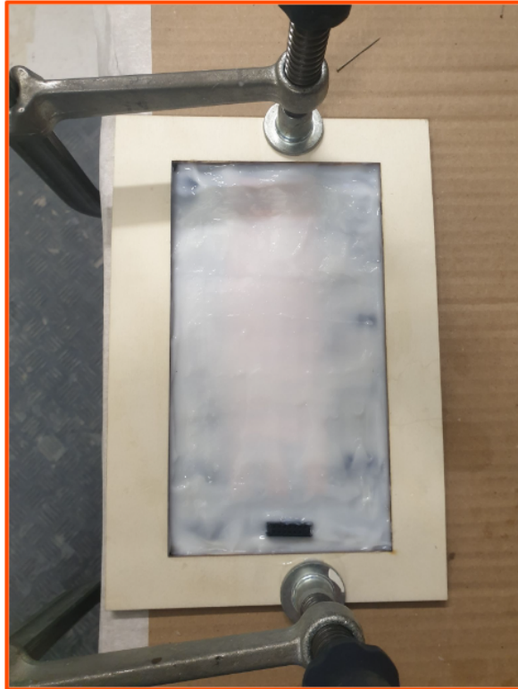
Figure 56: Setup of the third Trill prototype with silicone poured
