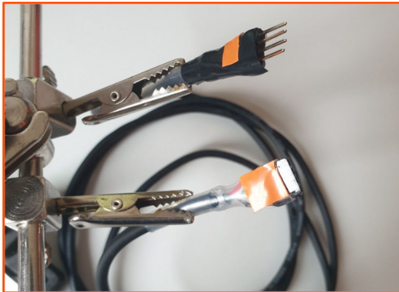
Figure 69: A cable for connecting the Trill and microcontroller
