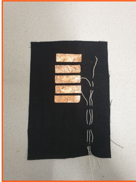
Figure 53: Piece of fabric with electrodes and embroidered wiring
