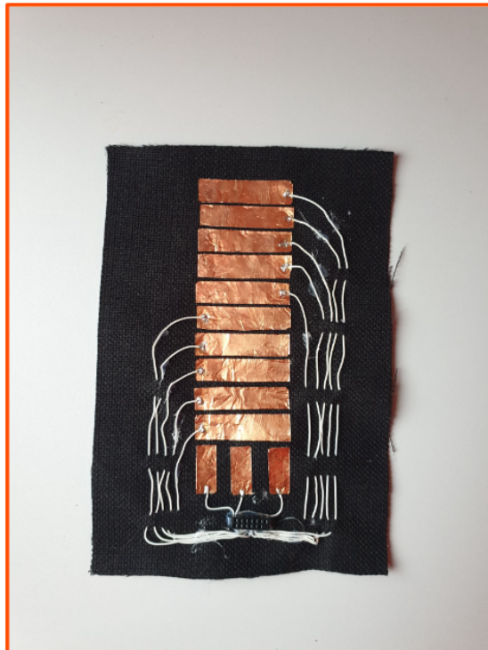
Figure 54: Piece of fabric with electrodes, embroidered wires and connector
