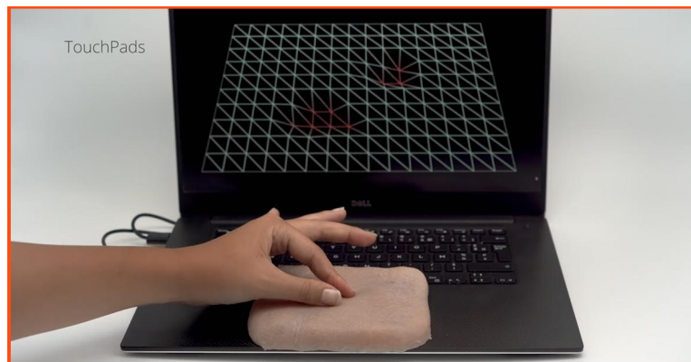
Figure 10: Artificial skin created by Marc Teyssier, showing how the skin can sense pressure and position
