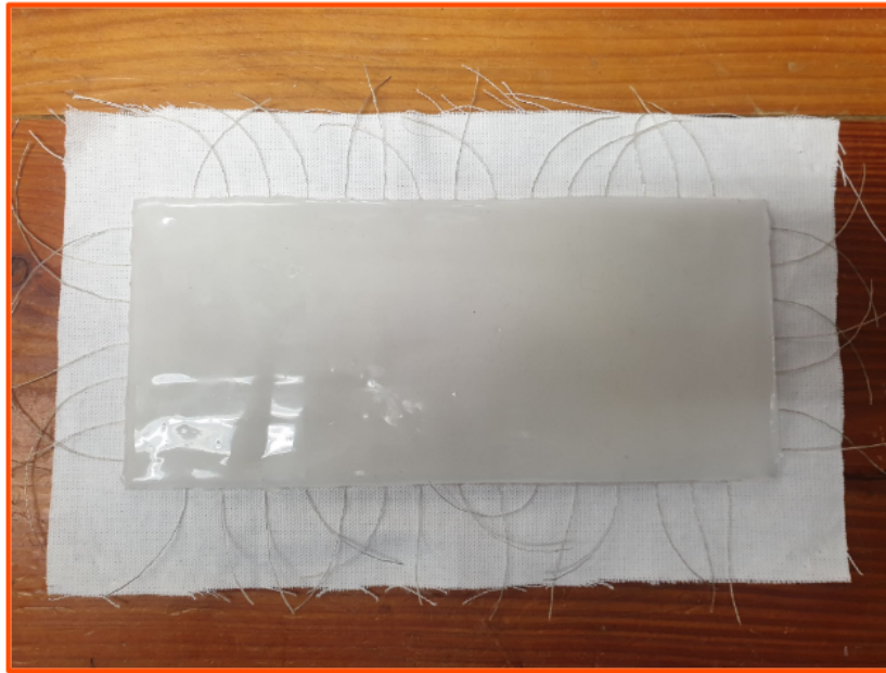
Figure 76: The piece of fabric with conductive thread electrodes and cured silicone
