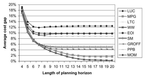
Figure 3.3: Average Cost Gap Between Scheduling Costs and Optimal Solution [1]
