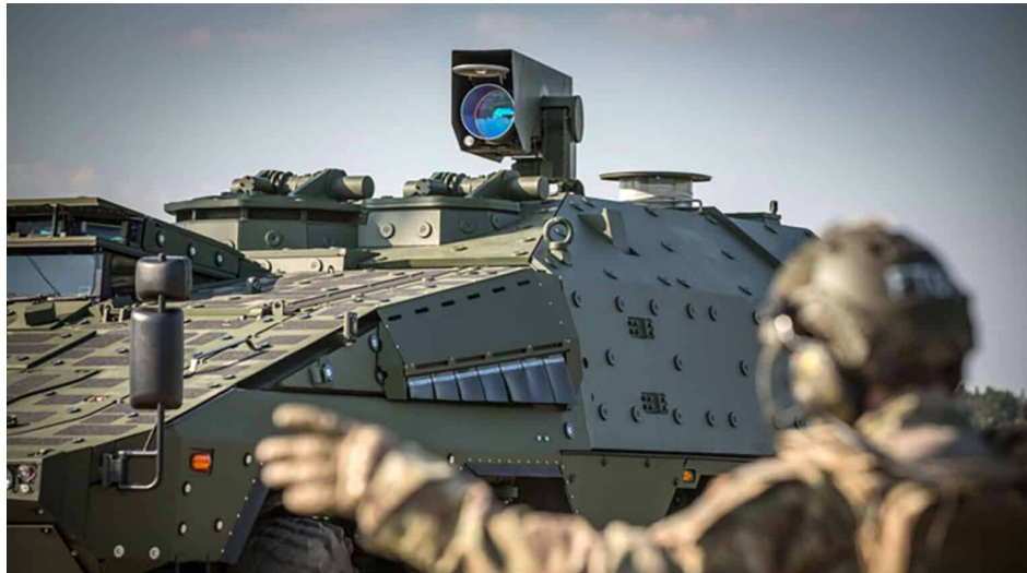
Figure 3.4: An example of a HEL module on the Boxer Infantry Fighting Vehicle [54]
