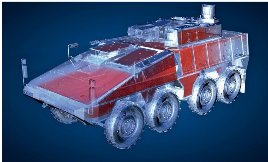
Figure 3.5: The composite armour of a Boxer Infantry Fighter Vehicle [55]
