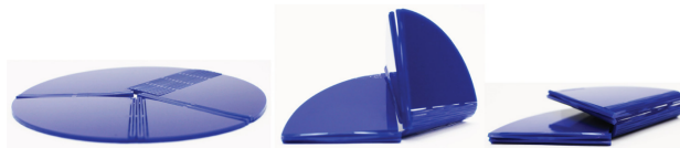
Figure 5: Example of the bending of a strained joint in three stages [9]
