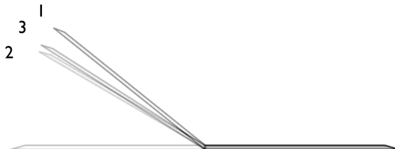
Figure 18: Undamped behaviour of the iteration process on a two panel origami.
