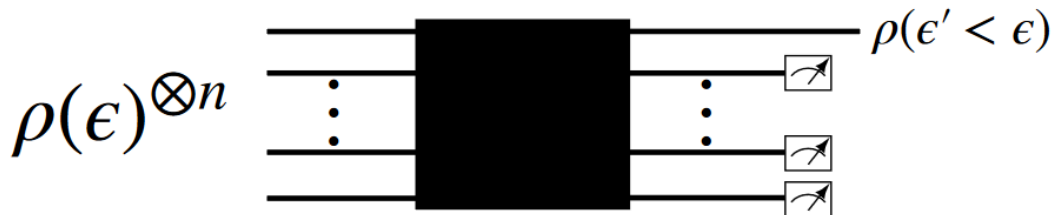
FIGURE 1: Illustration photon distillation experiment. N "copies" of photons with a state described by \rho(\epsilon) are sent into a N -mode interferometer of which N - 1 ancillary modes are measured. The \epsilon gives an indication for the error of the photon. The remaining photon has a state described by \rho(\epsilon') , such that \epsilon' < \epsilon . SOURCE: Distillation of Indistinguishable Photons . [11]
