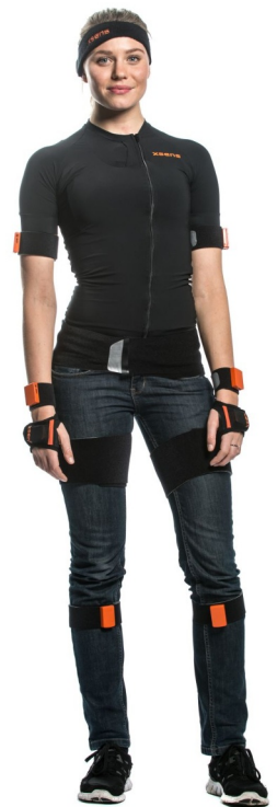
Figure 1: A woman wearing a set of MTw sensors [13]
