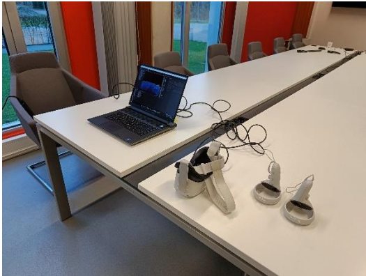
Figure 5. The set-up: the Alienware laptop is connected to the Oculus Quest 2 with a link cable
