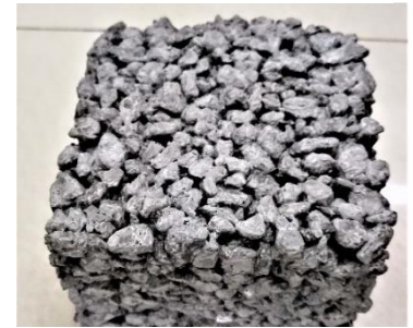
Figure 6.2 porous concrete. ((Chen & Chen, 2019)
