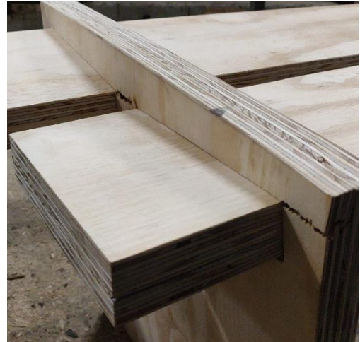
Figure 7.6 Structural failure 1:1 multiplex model
