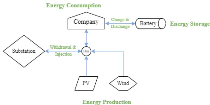
Figure 5: A Basic Energy Hub Configuration
