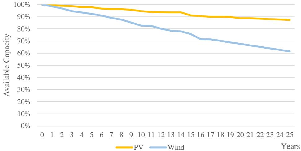
Figure 16: Technological degradation for renewable energy generators
