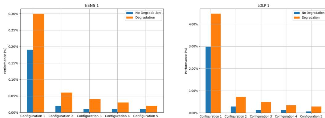
Figure 17: EENS and LOLP at Consumer 1 for each configuration variant
