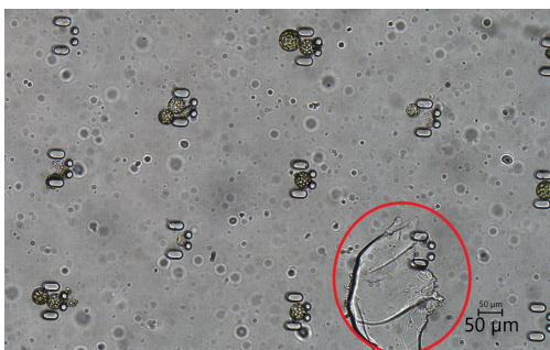
Figure 9: Picture of debris (inside of the red circle) in the chip.
