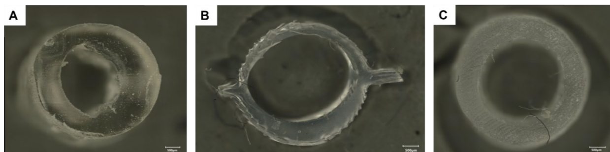
Figure 5-4: Microscopy imaging of circumferential slices of materials used for creating umbilical veins. A: Vascuflex, B: HT 33, C: Superflex. The scale bar at the bottom right represents 500 \mu\text{m} .
