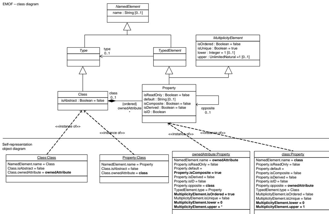
Figure 46 : Association between Class and Property as object diagram
