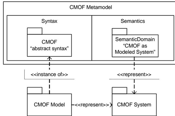
Figure 27 : CMOF as modeled system
