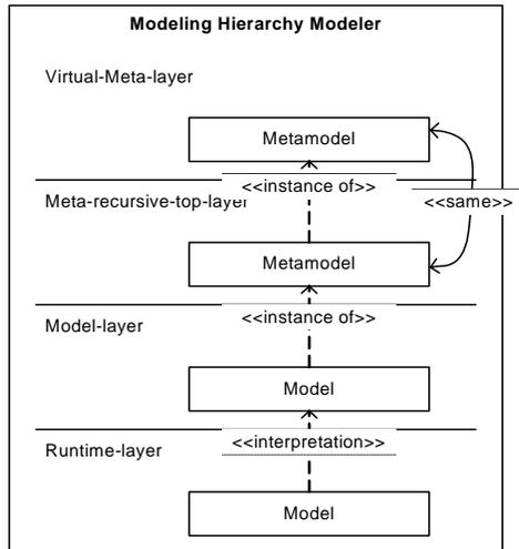
**Figure 14 : Self-representation through a virtual meta-layer**
