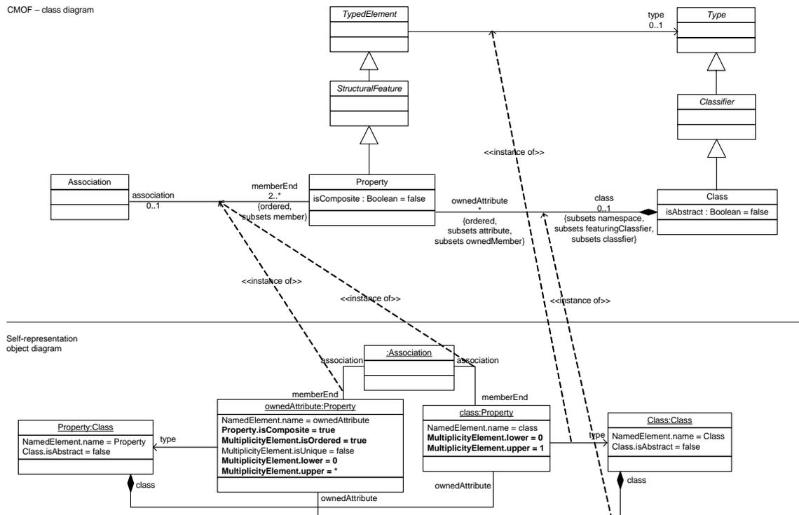
Figure 52 : Association between Class and Property as object diagram
