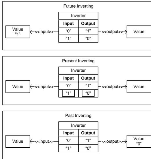
**Figure 11 : Runtime view of the inverter**
