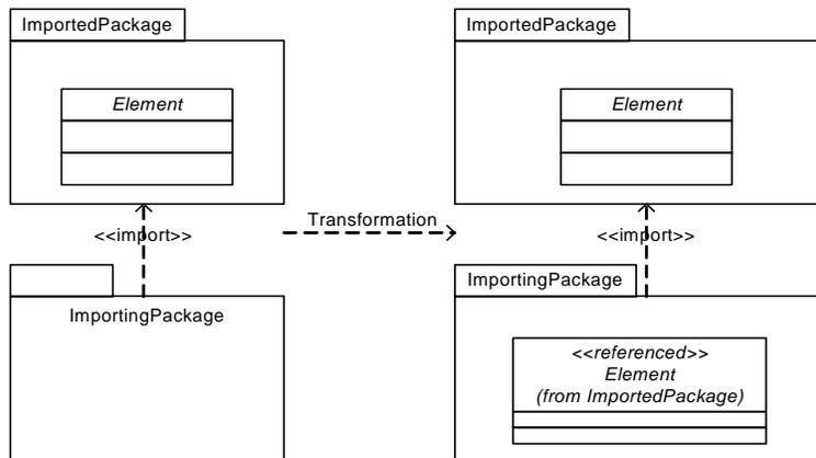
**Figure 30 : Transformation of packages according import**
