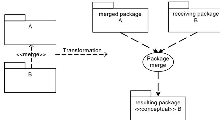
**Figure 31 : Transformation of packages according merge**
