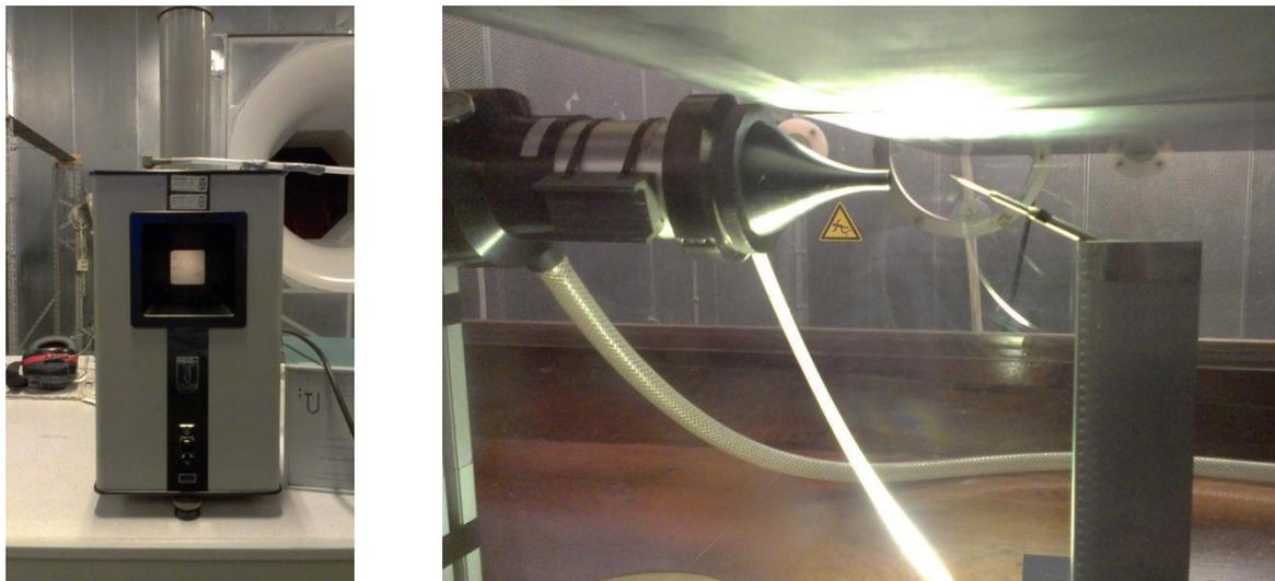
Figure 4.1 left: Betz manometer Right: Funnel with probe for calibration
