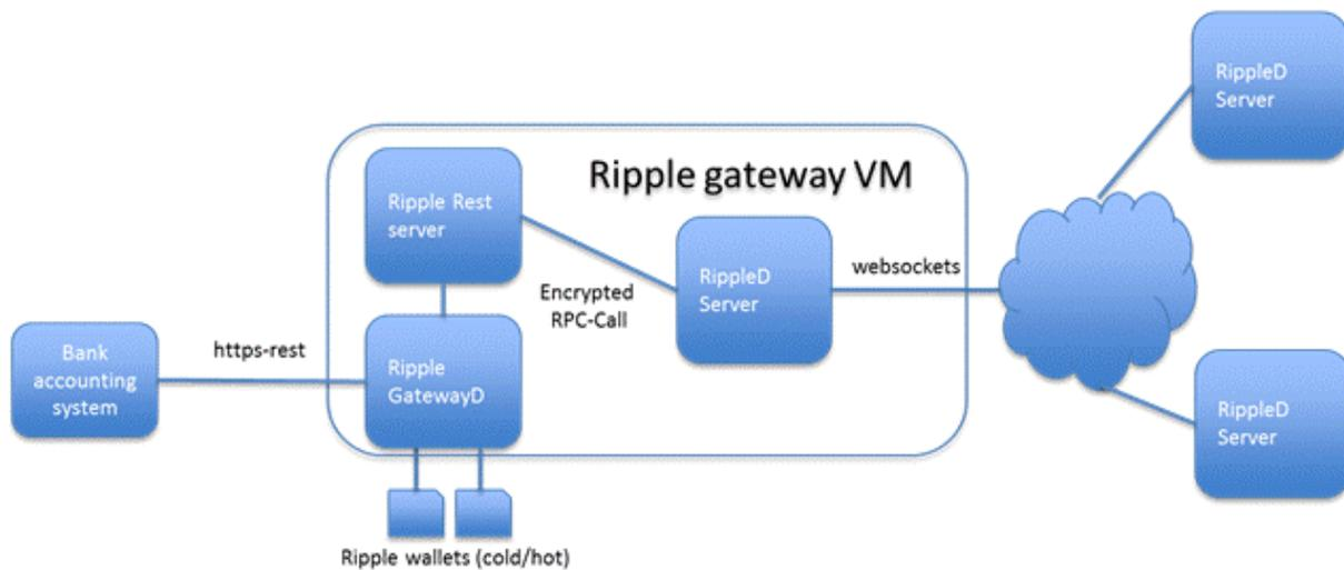
Figure 6.8 The Ripple technology linked to a banking system
