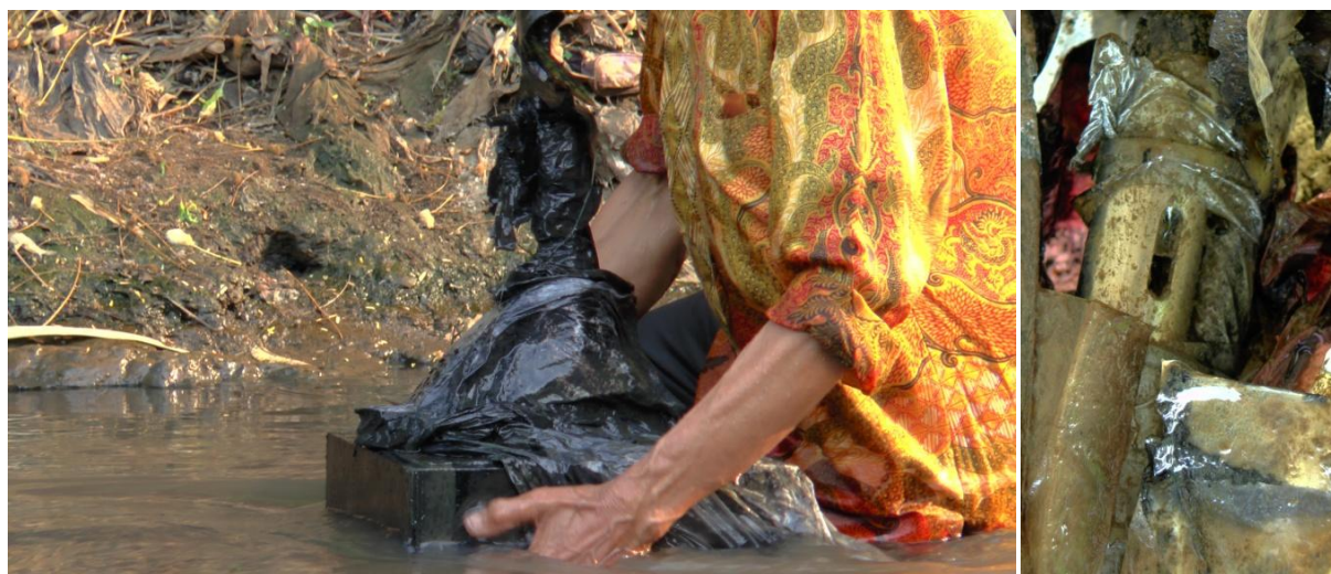
FIGURE 21 CLOGGING OF WASTE TO THE SENSOR AND ITS FRAME (LEFT) AND THE SENSOR HOLE (RIGHT) AT LOCATION 3 (22/5/2015)
