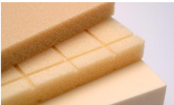
Figure 0.7: Panels of SAN foam, used as a core material in composite sandwich panels.
