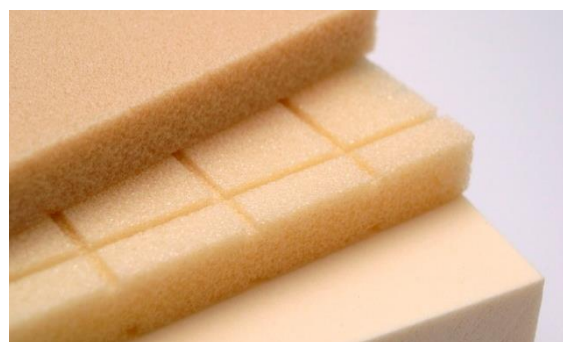
Figure 0.2: Panels of SAN foam, used as a core material in composite sandwich panels.
