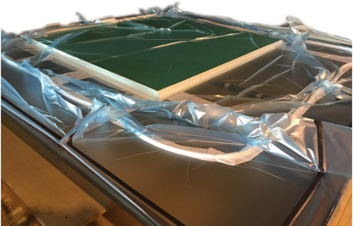
Figure 0.5: The vacuum infusion process; in the picture it can be seen that the laminate is under vacuum and ready for the infusion of the resin.
