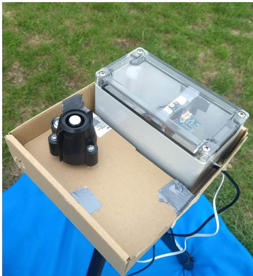
Figure 39: The test setup. Here you can see both pyranometers alongside each other.
