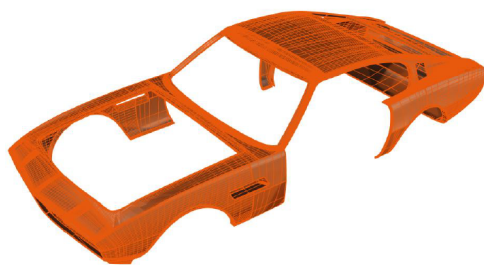
(a) Composite Body Buck Concept (Nedcam)
