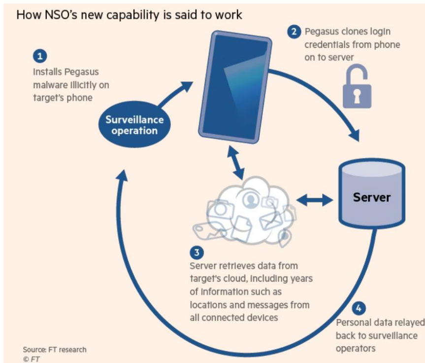
Image 1: The way Pegasus works on mobile devices. (Srivastava & Bradshaw, 2019).
