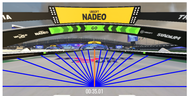
Fig. 8. The distance sensors are measurements from a point below the center of the image, to the walls of the track.
