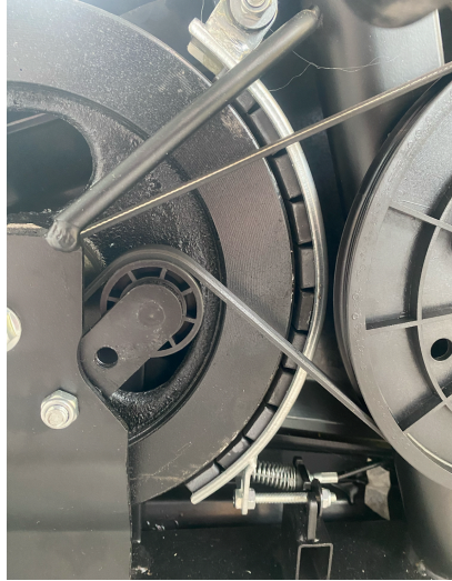
Figure 13: The brake mechanism on the hometrainer
