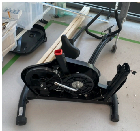
Figure 11: Exposed internals of the hometrainer
