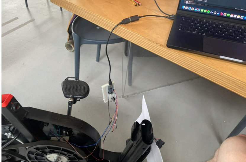
Figure 12: Prototyping with the hall effect sensor
