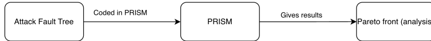
Fig. 2. The paper will take an AFT and write it manually into PRISM then extract the probabilities and create a Pareto front.
