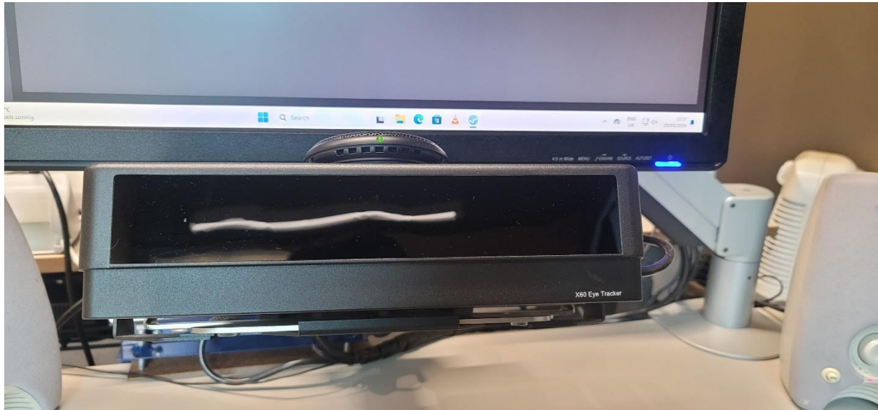
Figure 20: X60 Eye-tracker; used in usability study.
