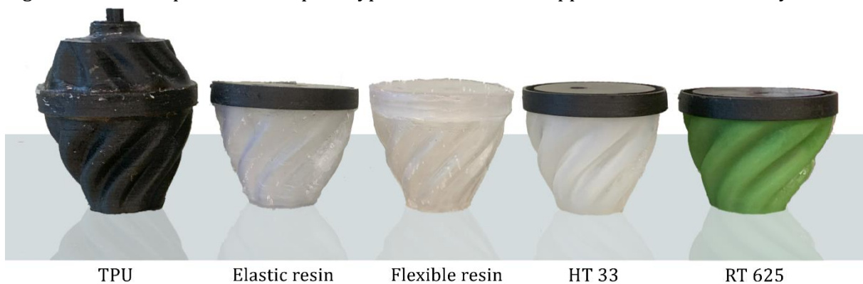
Figure 7-2: Prototypes of the different materials.
