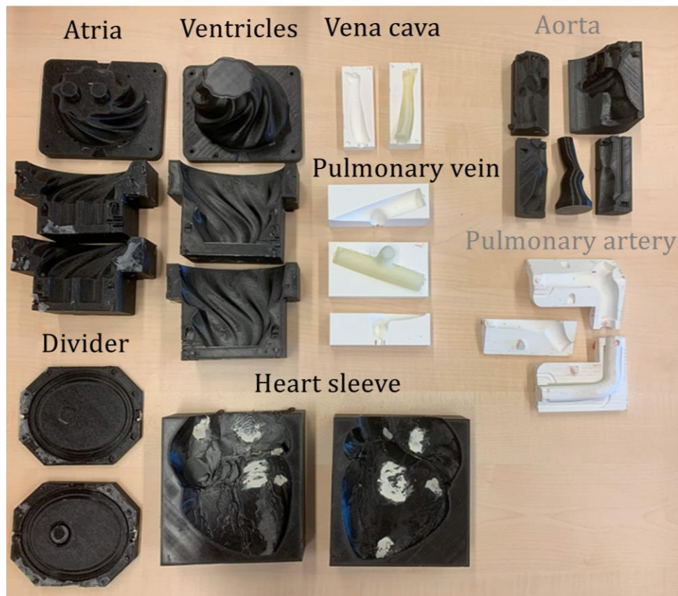
Figure 9-5: 3D printed moulds of the simulated heart parts. Black: new mould designs, Grey: moulds adapted and taken from De Jong [4].
