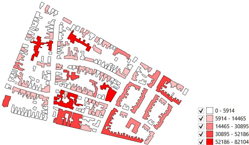
Figure 48 - Estimating Energy production per rooftop - in kWh.
