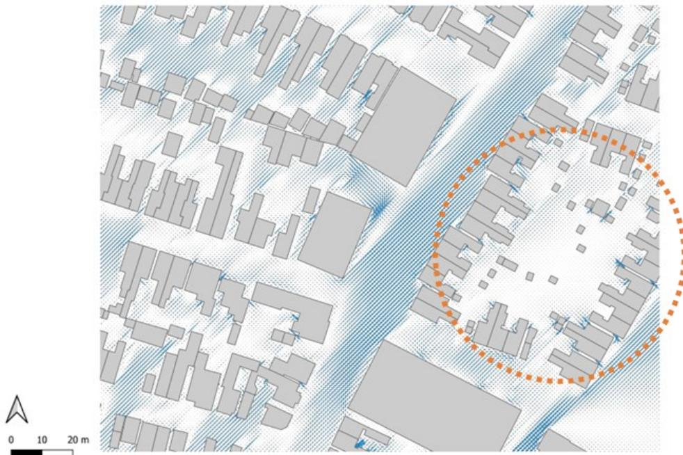
Map 14 - Wind Flow intensities on ground for Case C. There is considerable change in wind pattern observed due to introducing the tall building aligned E-W, which blocks wind effectively.
