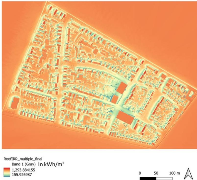
Map 5 - Estimation of Annualised Solar Irradiation values of the modified scenario with a cluster of Multiple Tall buildings – in kWh/m<sup>2</sup>
