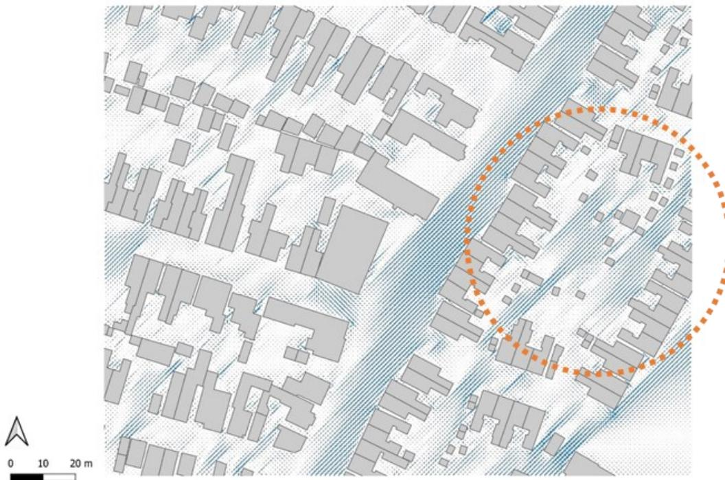
Map 12 - Wind Flow intensities on ground for Case B. Wind pattern is seen to be changing around the introduced tall building.
