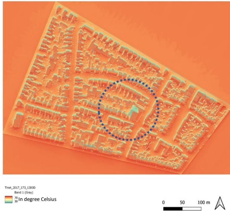
Map 17 - Tmrt - Mean radiant temperature estimate using SOLWEIG for Case B
