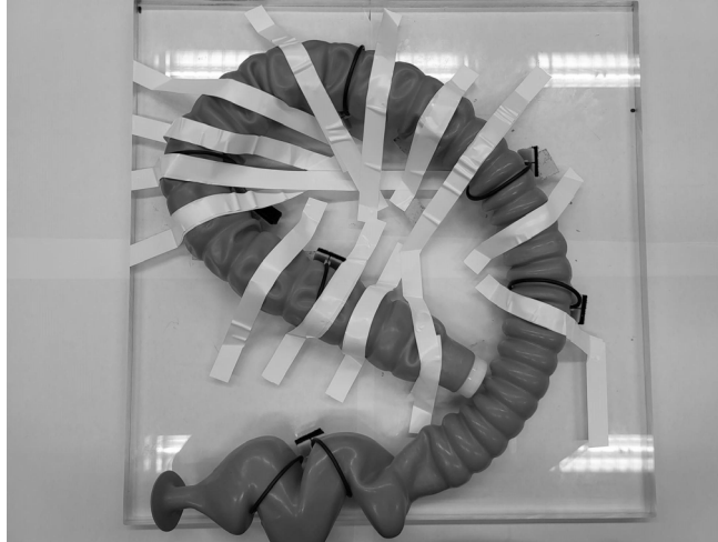
Figure 11: This is the taped down version of the Bowel Phantom. This was done to prevent the capsule from lifting the Bowel Phantom into the RPM. The tape was done in a way that prevents the Bowel Phantom from lifting into the RPM, while not constricting any of the haustra.
