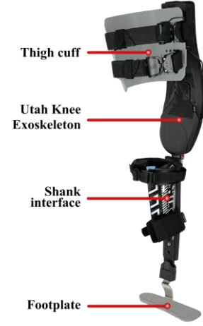
Fig. 1: A picture of the Utah Knee Exoskeleton, including covers and physical interfaces. A total of eight physically adjustable settings are present to improve fitting for a wider range of wearers.
