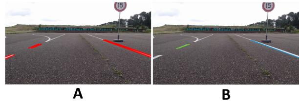
Fig. 10. Line fitting starting with Houghlines in A and the selected road lines in B.
