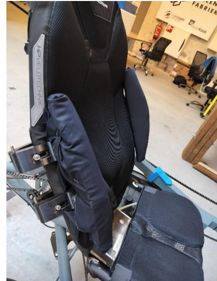
Figure 76: The final prototype with side bolsters, lumbar support and rotatable sitting area
