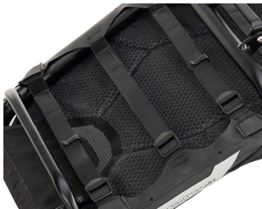
Figure 93: Velcro straps like on the HP-Velotechnik seat can also be used for a final concept
