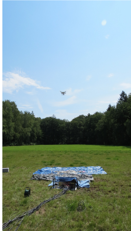
Figure 7.11: The field in which the measurements are performed. The UAV, acoustic camera, distribution boxes, and auxiliary equipment is visible.
