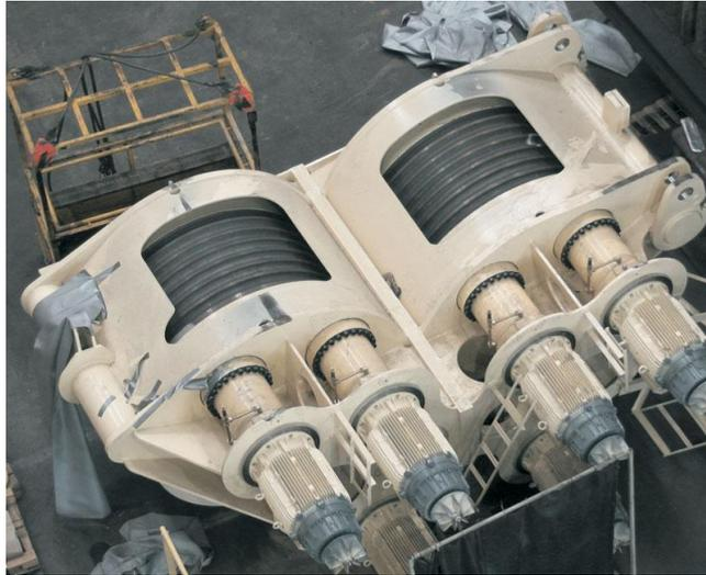
Figure 1.5: 2 Winches with electromotors with gears connected to the sides of the winch
