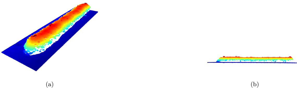
Figure 24: (a) Corner view and (b) side view of point cloud visualized using Open3D after removing outliers.
