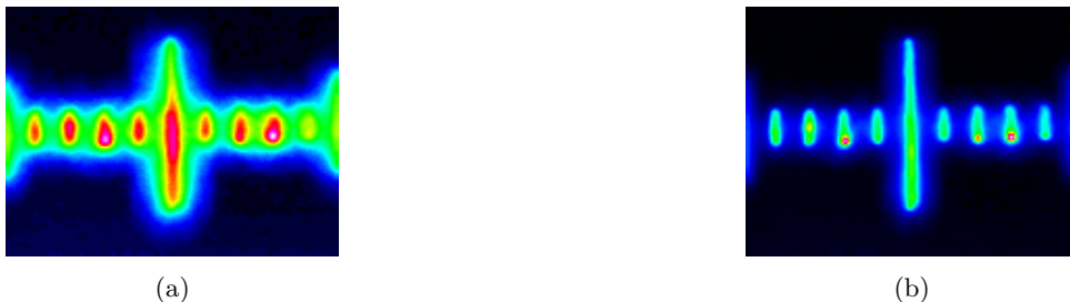
Figure 14: Colorized E-MAqS camera frames showing illuminated millimeter markings: (a) out of focus, and (b) in focus.
