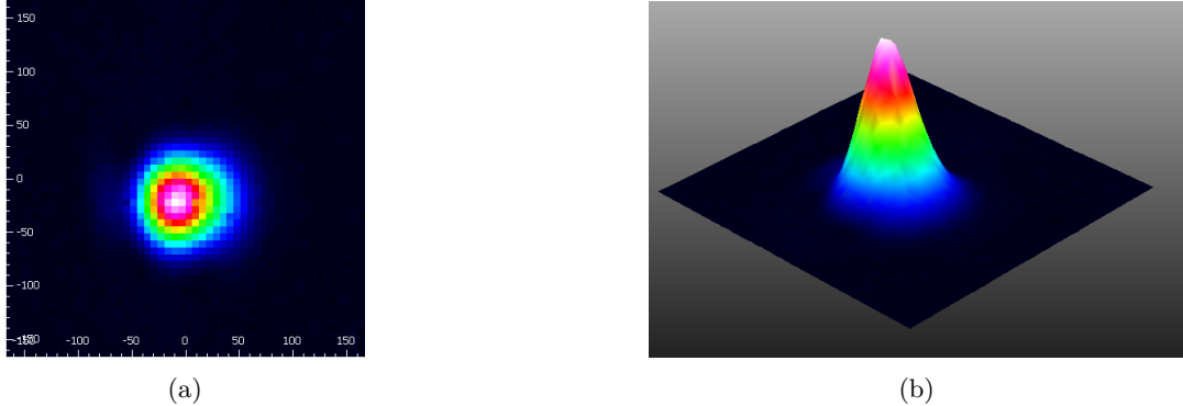
Figure 28: Beam profiling measurement of the OCT measurement beam in focus, depicted in (a) 2D with scaling in \mu\text{m} and (b) as a 3D surface.
