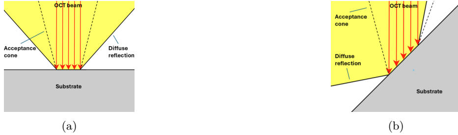
Figure 27: Schematic illustration of a diffuse reflection of the OCT measurement beam on a flat substrate (a) and on a 45^\circ angled substrate (b).
