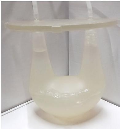
**Figure 34:** Fabricated BPE phantom with tumour in front view.
