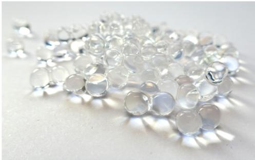
**Figure 9:** Sodium-Alginate beads, used to mimic the fine capillary network. [32]
