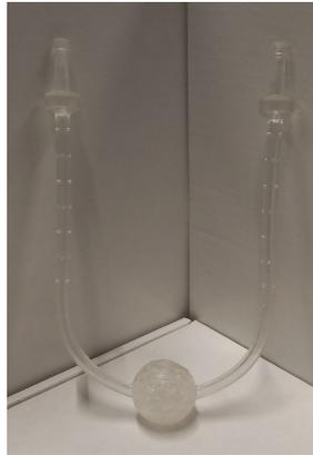
**Figure 33:** 3D printed tumour tubing.
