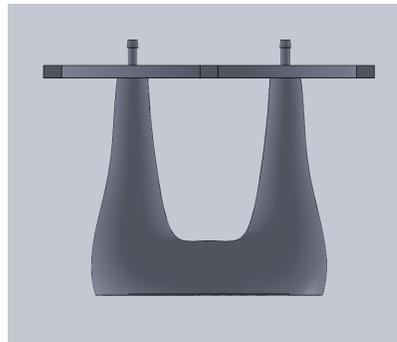
**Figure 21:** Upper part fillable BPE phantom in front view.
