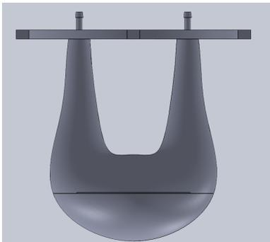
**Figure 20:** Total fillable BPE phantom in front view.
