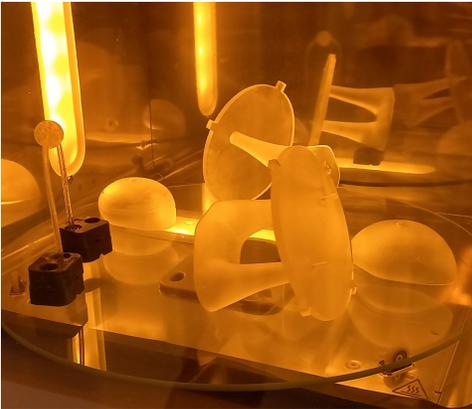
**Figure 32:** New fillable BPE phantom and BPE phantom with tumour curing in the FormLabs Form Cure L.
