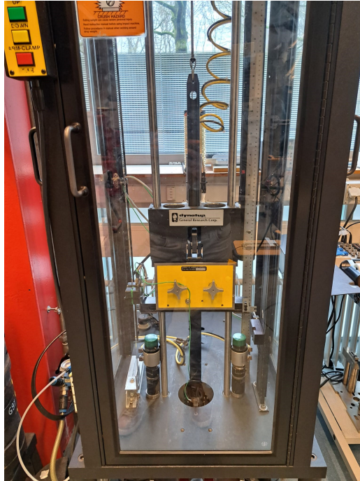
Figure 4.1: Dynatub drop weight impact tower setup used at the facilities of UTwente
