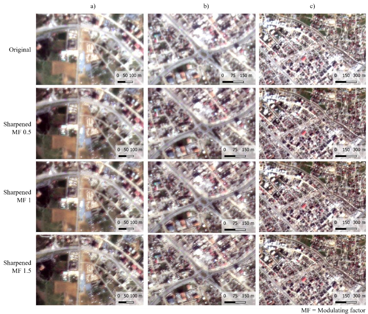
Figure 27. Visual comparison of PS images sharpened by a post-event Pleiades image using modulation factors for Nurdagi (AOI 3) showing (a) temporary shelters, (b) road cross-section and debris pile, (c) buildings.
