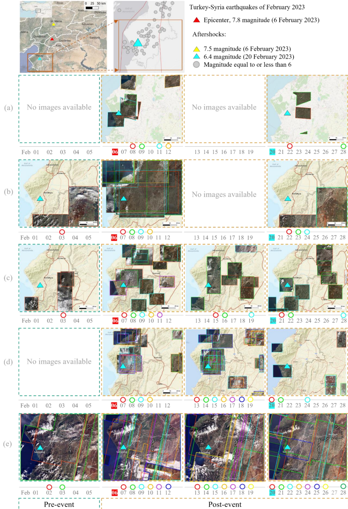
Figure 3. Pre- and post-event data availability from different high-resolution satellite data sources for the Kahramanmaraş earthquakes that occurred on 6th February 2023. The scene covers the province of Hatay from Türkiye and its surrounding region spanning an approximate area of 7800 km 2 that experienced several aftershocks with the highest magnitude of 6.7. (a) WorldView (0.3 meters), (b) SPOT (1.5 meters), (c) Pleiades (0.5 meters), (d) Pleiades Neo (0.3 meters), (e) PlanetScope (3 meters).
