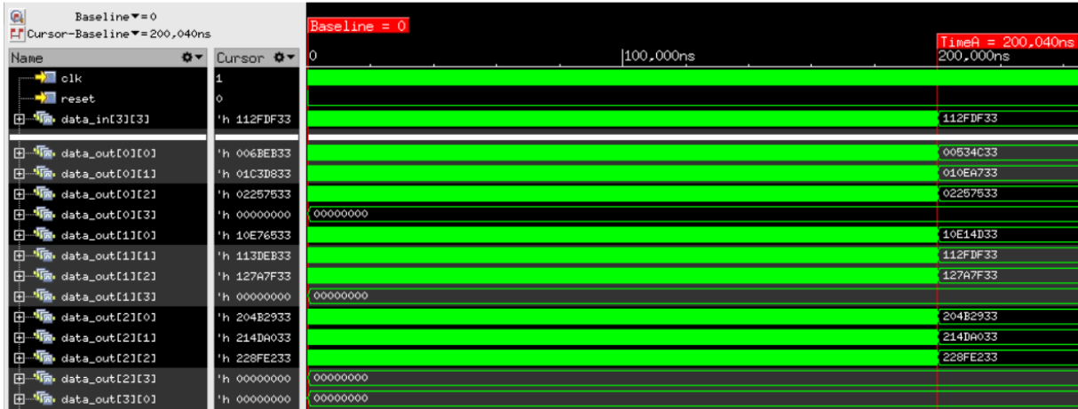
Figure 6.9: Waveform of inserting 100,000 directional packets into node (3,3)
