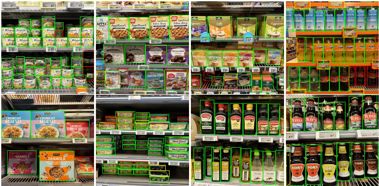
Figure 9: Prediction results of product detection on Grocery Products [13], WebMarket [14], and Dutch Markets datasets. Green boxes indicate correct detections (true positives), yellow boxes represent false detections (false positives), and red boxes highlight ground truth objects that were missed by the model (false negatives).
