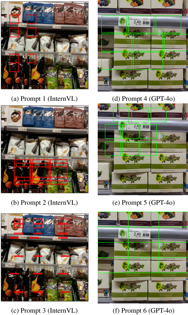
Figure 10: Comparison of object grounding results using six different prompts. The left column shows results from InternVL2.5 [53] (Prompts 1–3), while the right column shows results from GPT-4o [54] (Prompts 4–6). Red and green bounding boxes indicate the detected product regions by InternVL2.5 [53] and GPT-4o [54], respectively.
