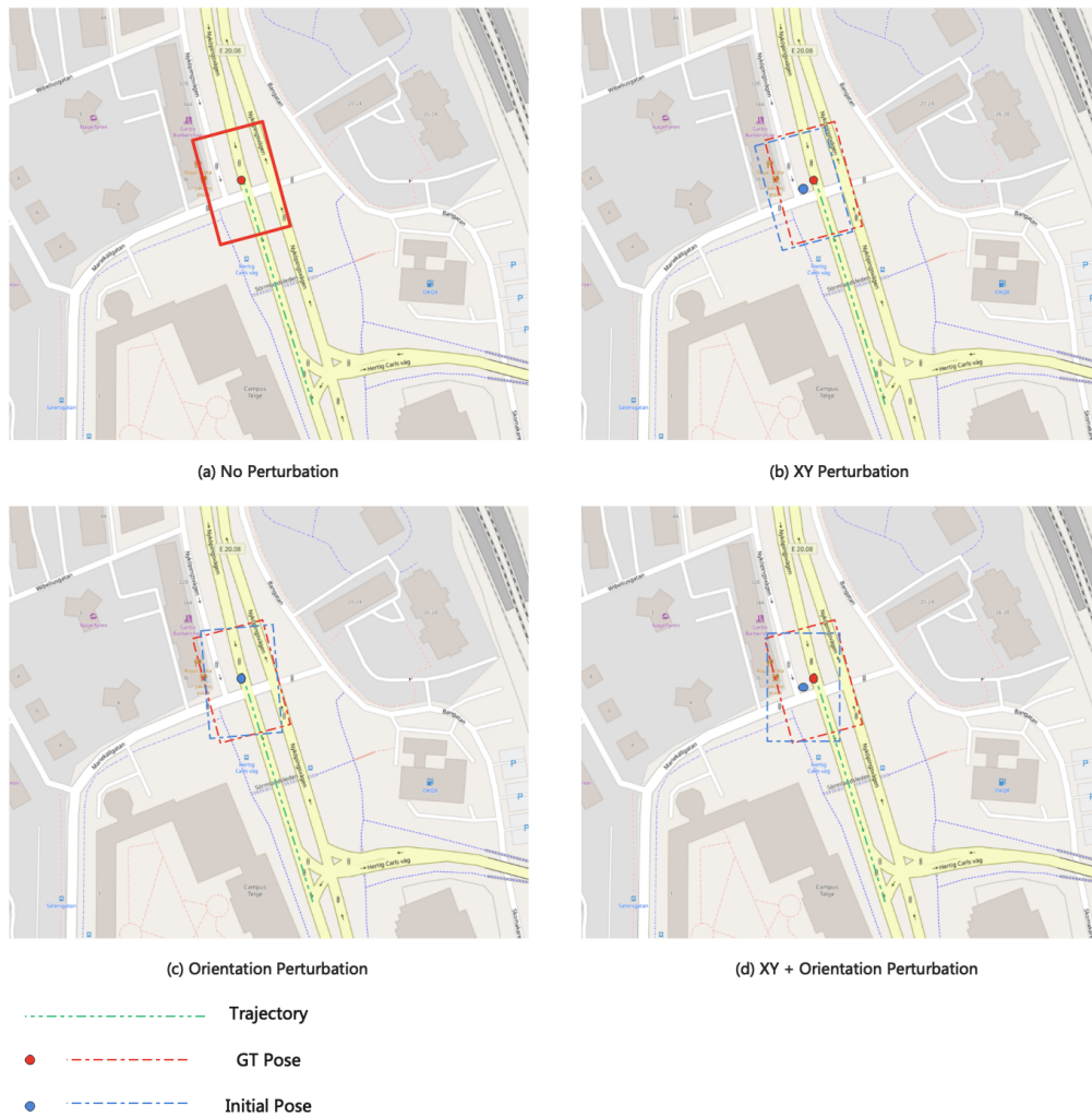
FIGURE 4.1: Comparison of localization robustness under different initial pose perturbation scenarios: (a) no perturbation, (b) XY translation perturbation, (c) orientation perturbation, (d) combined perturbation (translation + orientation).
