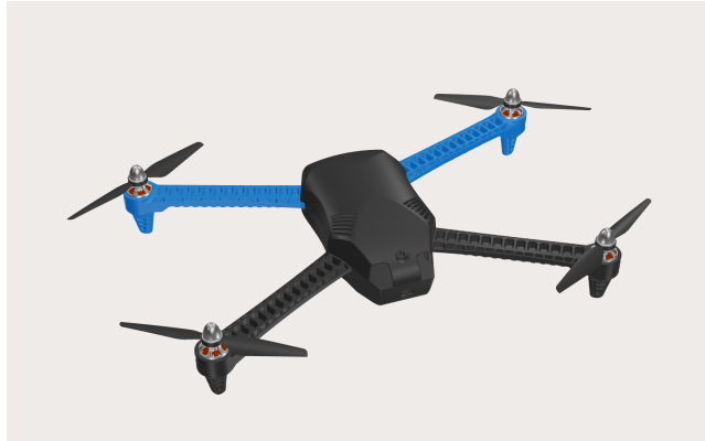
Figure 4.7: 3DR Iris UAV used in Isaac Sim [86]
