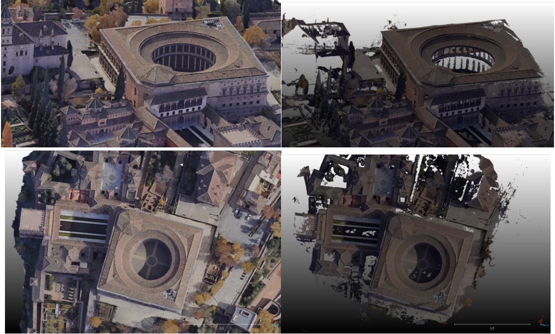
Figure 5.20 Ground truth (left) and the reconstructed point cloud (right) for the building
